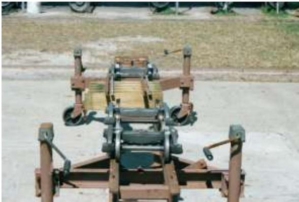
LCRR provided a table with screw jacks at the four corners so that the table may be tilted. Picture # 1 shows the tilting table with the screw jacks and with three trucks on it.
