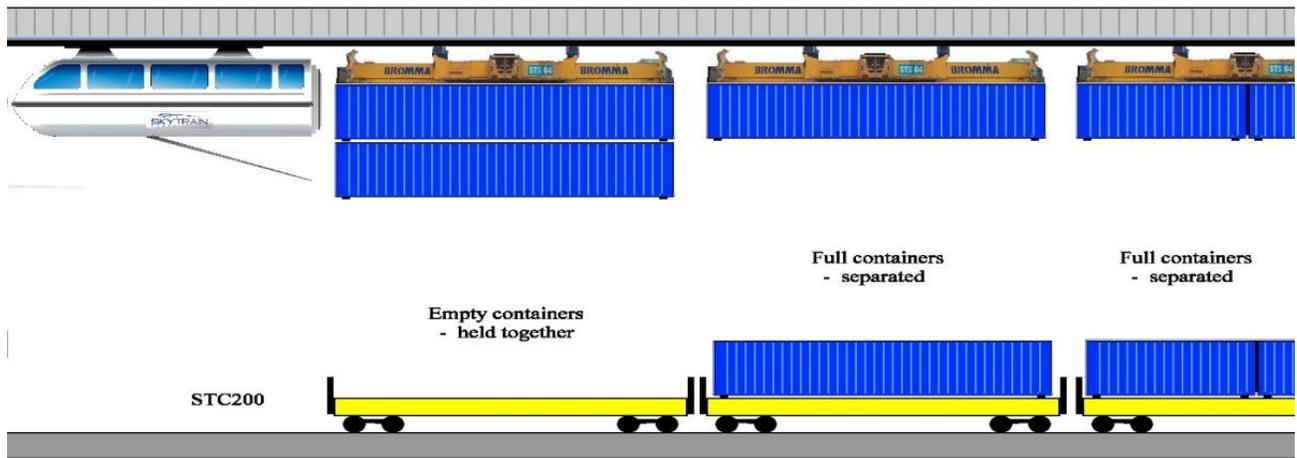
As shown below (showing the loading of a ship), STC envisions a fleet of Enhanced automated self-propelled rail-carried flatcars, labelled "STC200", moving individually in a circulatory fashion between the container handling cranes and transfer points, where the containers could be transferred to/from Stackers or beam carried vehicles, labelled "STC150".
