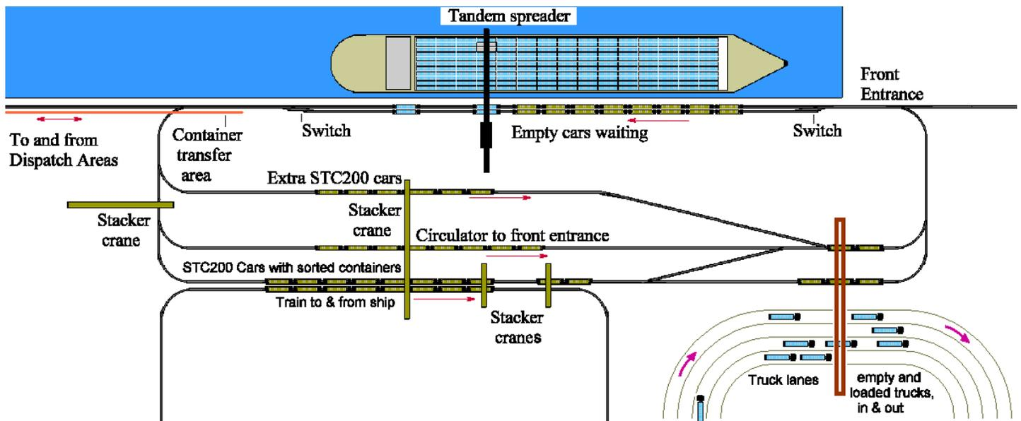
The track along the pier will consist of a rail with the following sections (from right to left):
