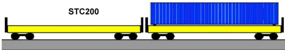
As shown below (illustrating the loading of a ship), STC envisions a fleet of Enhanced automated self-propelled rail-carried flatcars, labelled “STC200”, moving individually in a circulatory fashion between the container handling cranes and transfer points, where the containers could be transferred to/from Stackers or beam carried vehicles, labelled “STC150”.
