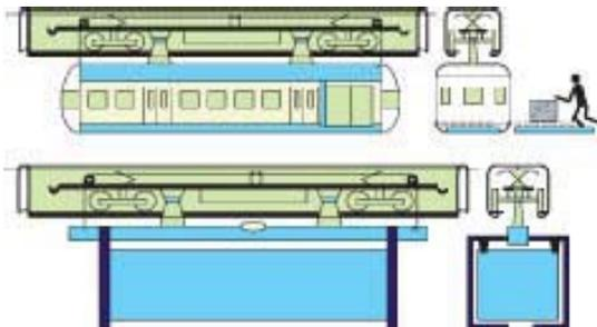
Combination car adapted for automated small container loading on the top left. The vehicle has a movable floor to become a wall allowing automated small freight loading for off peak times gaining extra revenue removing trucks from the roads.
